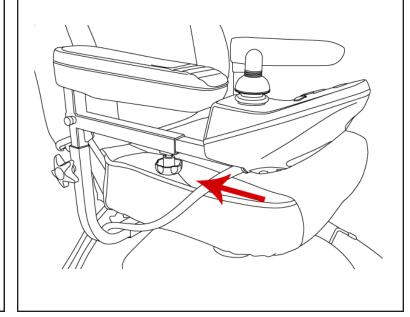
Connect the main cable from the controller to the connection port in the product's cover shroud.
