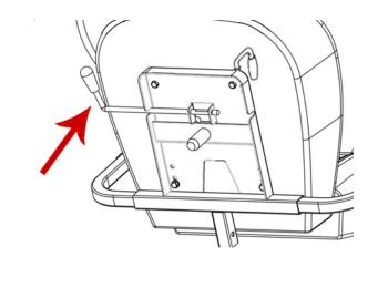
Insert the armrests into the attachment, in the seat frame so that the armrests face
