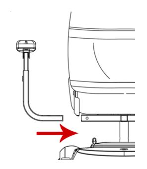
Insert and tighten the included star knobs to lock the armrests into place at the desired width.
