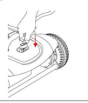
Fully charge the wheelchair's batteries by inserting the round charger connector into the battery charging terminal on the front of the wheelchair's controller and inserting the 3-pronged plug into a standard electrical outlet.
