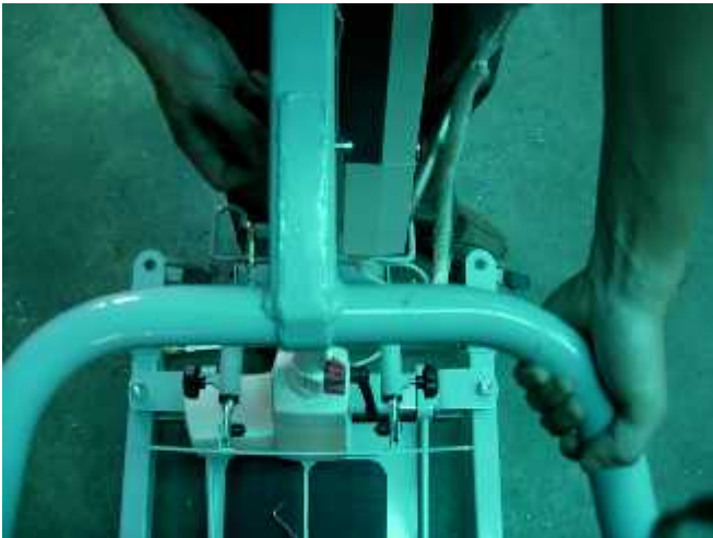
Install bottom actuator bolt thru lift and actuator.
